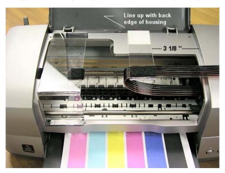
Use a pencil or marking pen, and mark a line on the printer housing, at 3 1/8 inches from the edge of the printer housing as shown in the above photo. *This photo was taken after the tubes were installed.*
